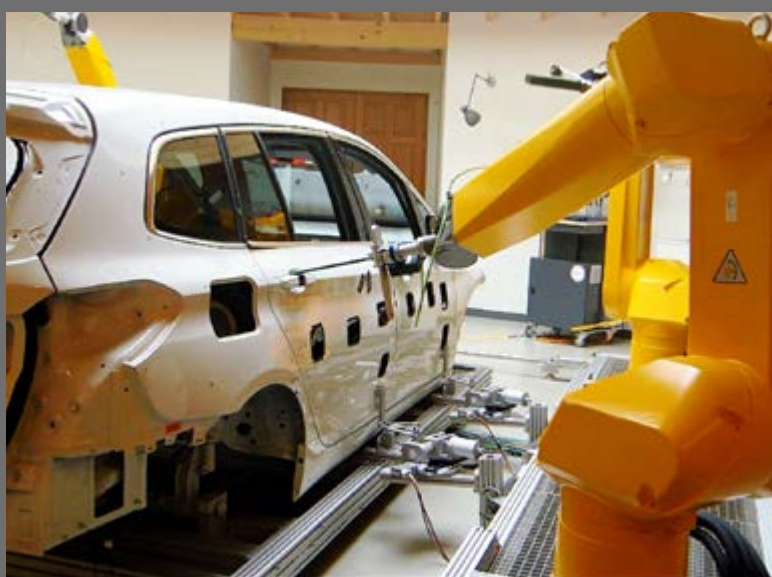
Tools greifen an Türe an / Tools engage the door
